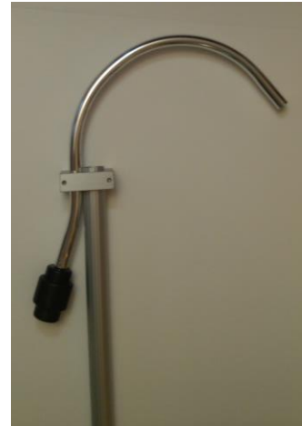
Shepherd's hook exhaust collector with telescopic pole for vertical exhausts
